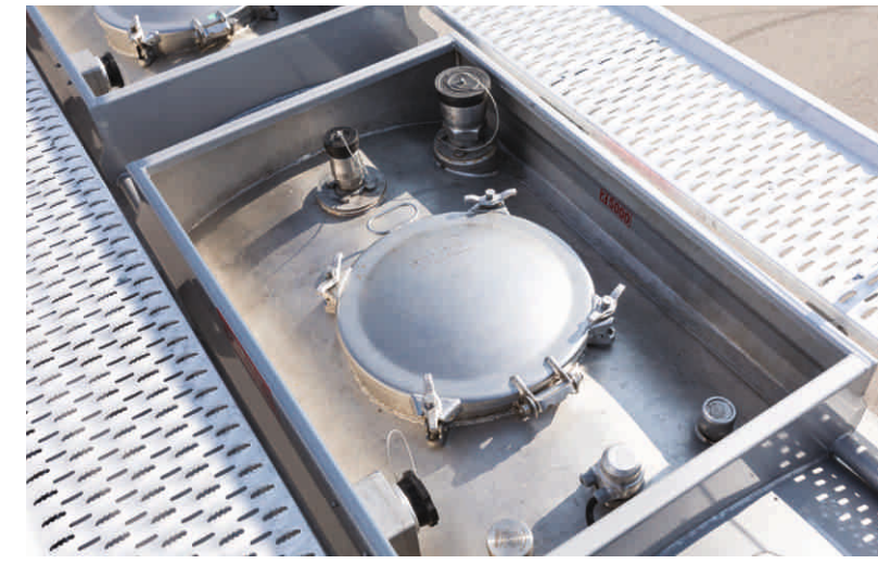
Spilltrays type top pool Protect armatures against possible rollover and impact
