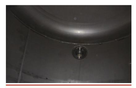
**Transverse seamless monolithic plates in the body structure** The least number of (T) joints provide high strength and long life
