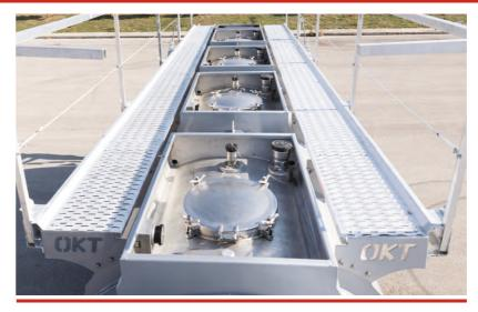
Two sides and automatic opening guardrail Provides ease of use, safety and automatically locks the brake system
