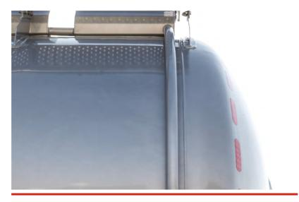
Seamless high performance robotic welding technology Minimizes welding faults on the body due to tension and human factors and secures against impact
