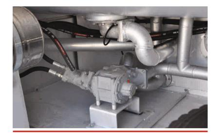
**Optional Pump-Driven Discharge System**Ergonomic handling with optimized hydromotor, piping and technical equipment provides fast and high flow rate discharge
