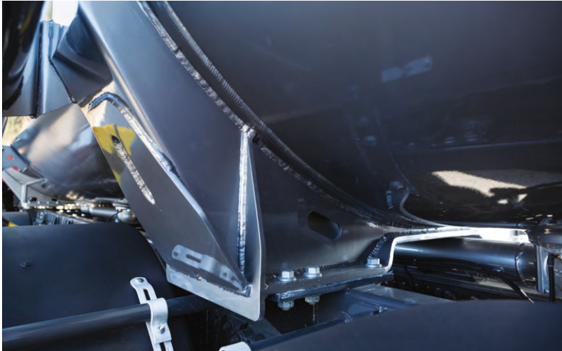
OMEGA mounting slots and tension relief cavities on the chassis Perfect fit between body and chassis under all kinds of road conditions, increase strength, reduce tension by distributing coming to the body force.
