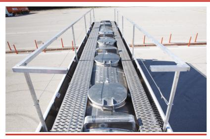
**Two sides and automatic opening handrail** Provides ease of use, safety and automatically locks the brake system
