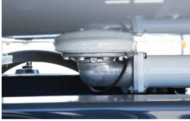
Outputs opened by deep drawing method At the bottom of the tank, it provides full discharge of the product.
