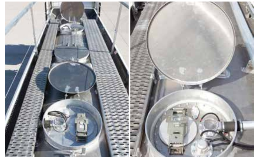
Built-in type manhole covers Protect armatures against possible rollover and impact. Protective cover The equipment on the manhole cover is protected against seasonal weather conditions (rain, snow, sun, dust)
