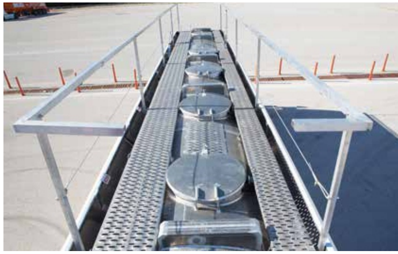
Two sides and automatic opening handrail Provides ease of use, safety and automatically locks the brake system.
