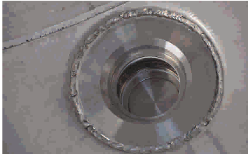
Bottom discharges opened by deep drawing method Provides full discharge of the product at the bottom of the tank
