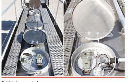
**Built-in type manhole covers**Protect armatures against possible rollover and impact
