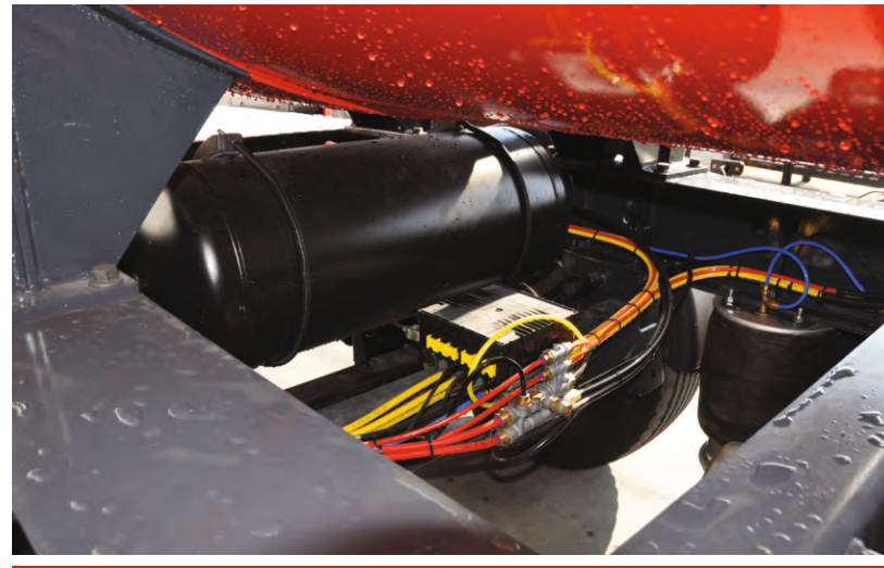
Coloured, POLYAMID air hoses Prevents complexity on installation cables, provides serviceability
