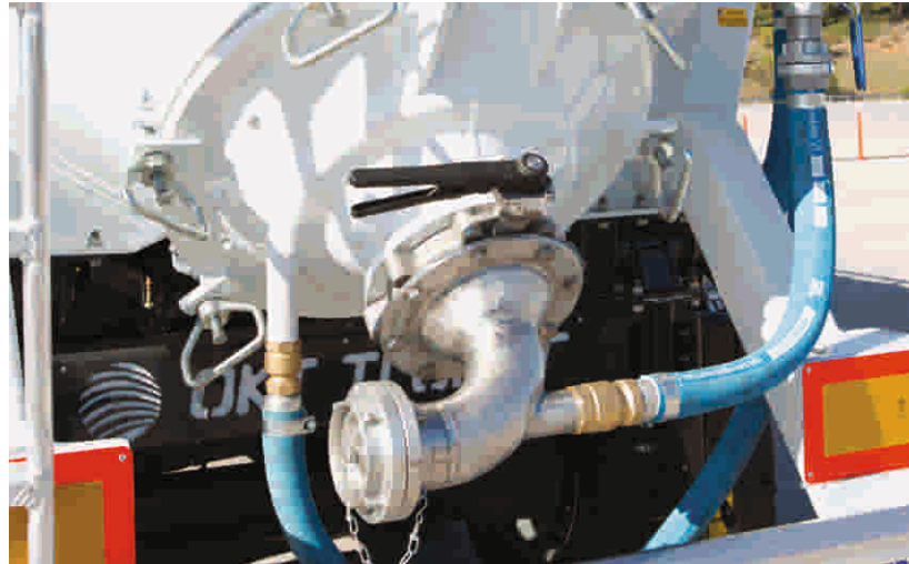
Outputs on the discharge funnel Pneumatic controlled, ergonomic, interceptible
