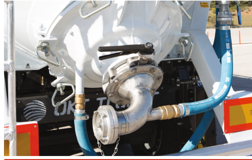
Outputs on the discharge funnel Pneumatic controlled, ergonomic, interceptible
