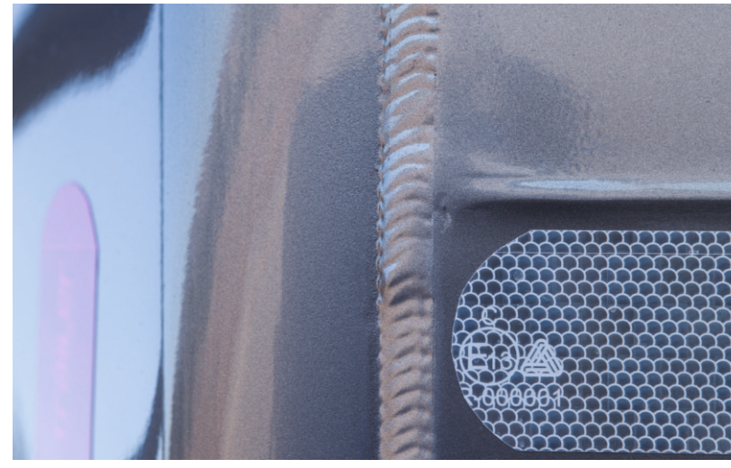
Seamless one-piece plates in the body structure The least number of (T) joints provide high strength and longlife
