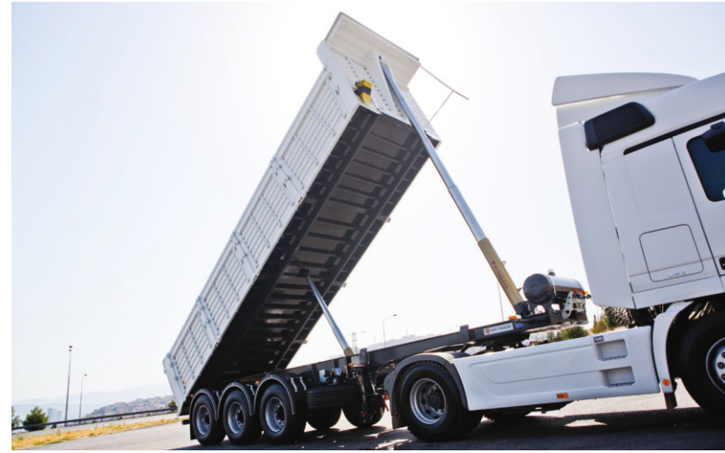
Hydraulic System Provides the discharge angle, emptying quickly and easily
