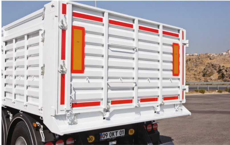
Self and side opening rear cover Facilitates material flow during unloading
