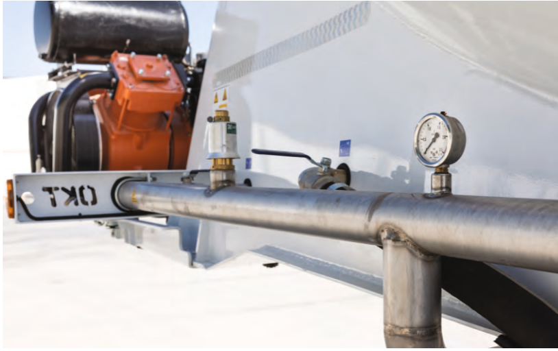
Safety valve and manometers Provides safe pressure control
