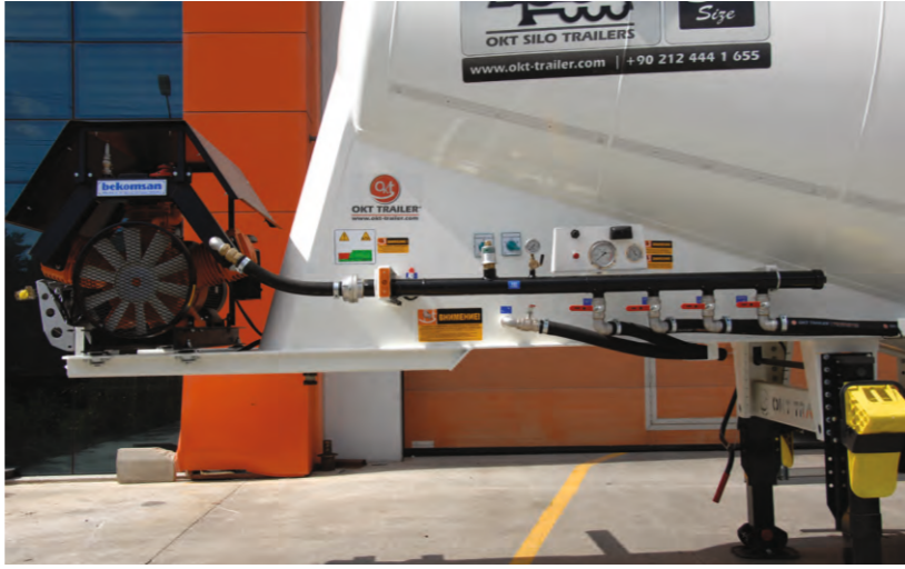
Grouped, defined and systematic drain line installation Ergonomic, easy accessible, controlled and rapid intervention
