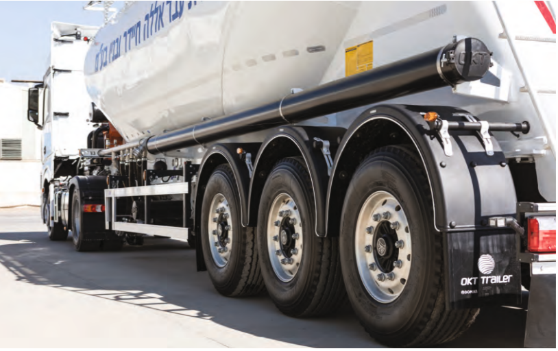
Integral construction on body and chassis Perfect fit between body and chassis under all kinds of road conditions, increase strength, reduce tension by distributing force to the body
