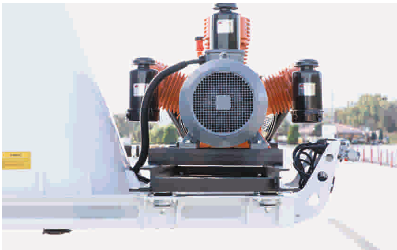
Portable compressor mounting platform Vibration absorber, Light and Strong
