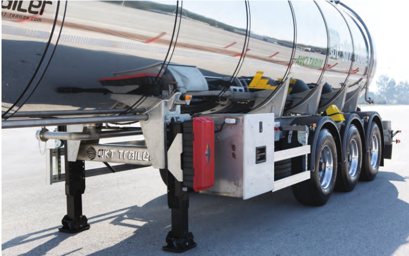
Sloping chassis design Provides complete discharge without any liquid remaining in the tank body
