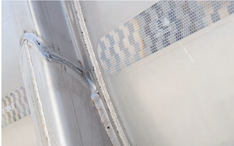
Use of robotic welding technology in OMEGA® monoblock connection saddles Increases body strength at chassis joints, reduces tension effect, provides unity of body
